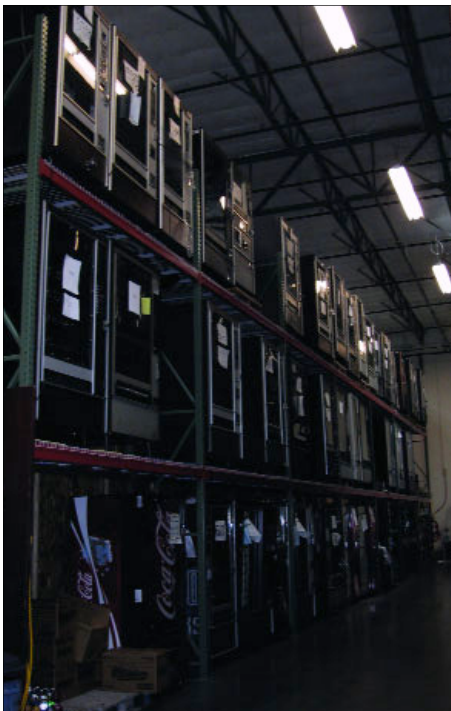
THREE UP: Courtesy Vending's three-high pallet racks for product and machine inventories makes efficient use of warehouse space.
